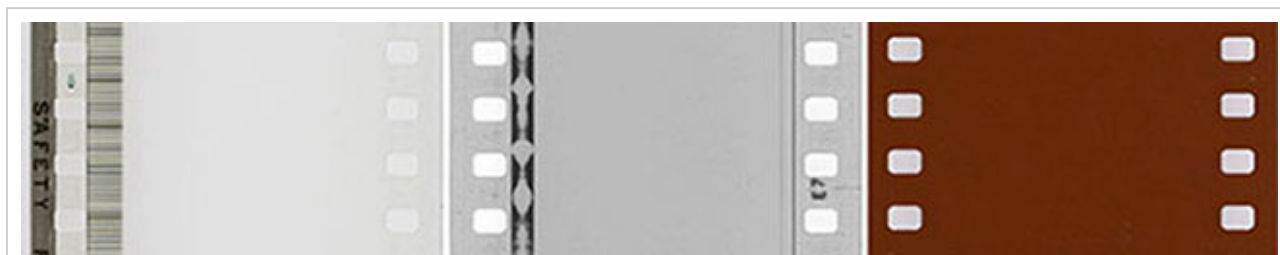
Examples of common soundtracks: a variable density optical track, a variable area optical track, and a full coat magnetic track.
